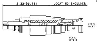
Direct-acting relief cartridges are normally closed, pressure-limiting valves used to protect hydraulic components
